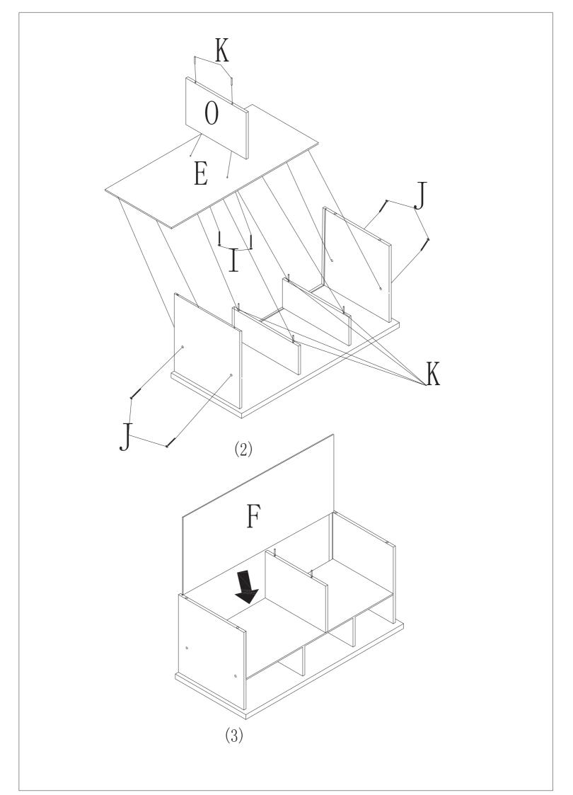
NOTE: THE BACK (F) MUST BE SEATED INTO THE GROOVE ON THE THE BOTTOM (A) OR THE TOP (G) WILL NOT FIT PROPERLY. LOOSEN AND RETIGHTEN THE PANELS IF NEEDED SO THAT THE BACK (F) IS FITTED INTO ALL GROOVES PROPERLY AND
